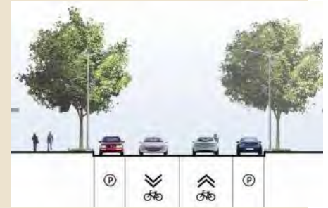
A sharrow is a travel lane shared by bicycles and other vehicles.
